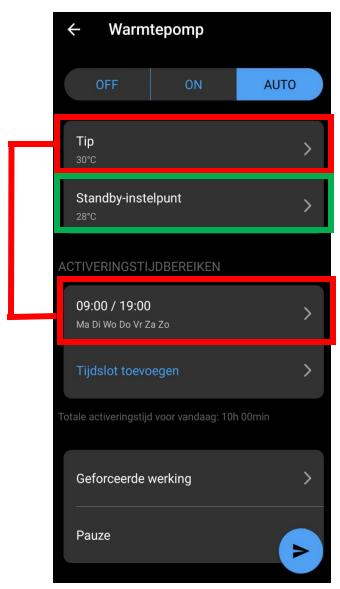
FYI: Keep in mind that the software will always take a margin of 1°C on the requested TIP temperature to prevent the heat pump from activating every tenth of a degree. So in this case, TIP 30°C will be about 31°C in practice
