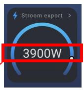
This indicates how much energy is put into the grid in the event of an overproduction of solar panels. Based on this value Smart Energy will activate the heat pump
