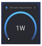
This indicates how much power is being imported from the grid for the whole house. This value is zero (or 1) when there is overproduction.
