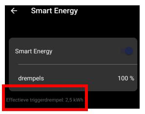
If you activate Smart Energy, you can set a threshold from the number of watts of overproduction that your heat pump will start for at least 30 minutes.
