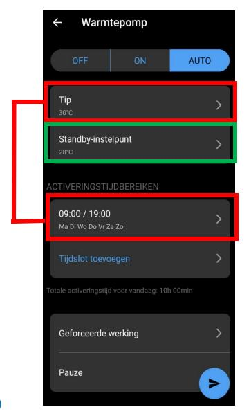
Note: Keep in mind that the software will always take a margin of 1°C on the requested TIP temperature to prevent the heat pump from activating every tenth of a degree. So, in this case, the 30°C TIP will be around 31°C in practice
